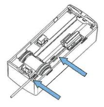
Return the heat cost allocator and plug the connector of the remote sensor into the interface inside the heat cost allocator
